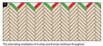
• all expansion wedges remain in their position. • all joints are closed and the strips are locked into one another.
