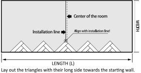
Align the center triangle top with the installation line. Make sure the underlay material is installed beforehand and the
